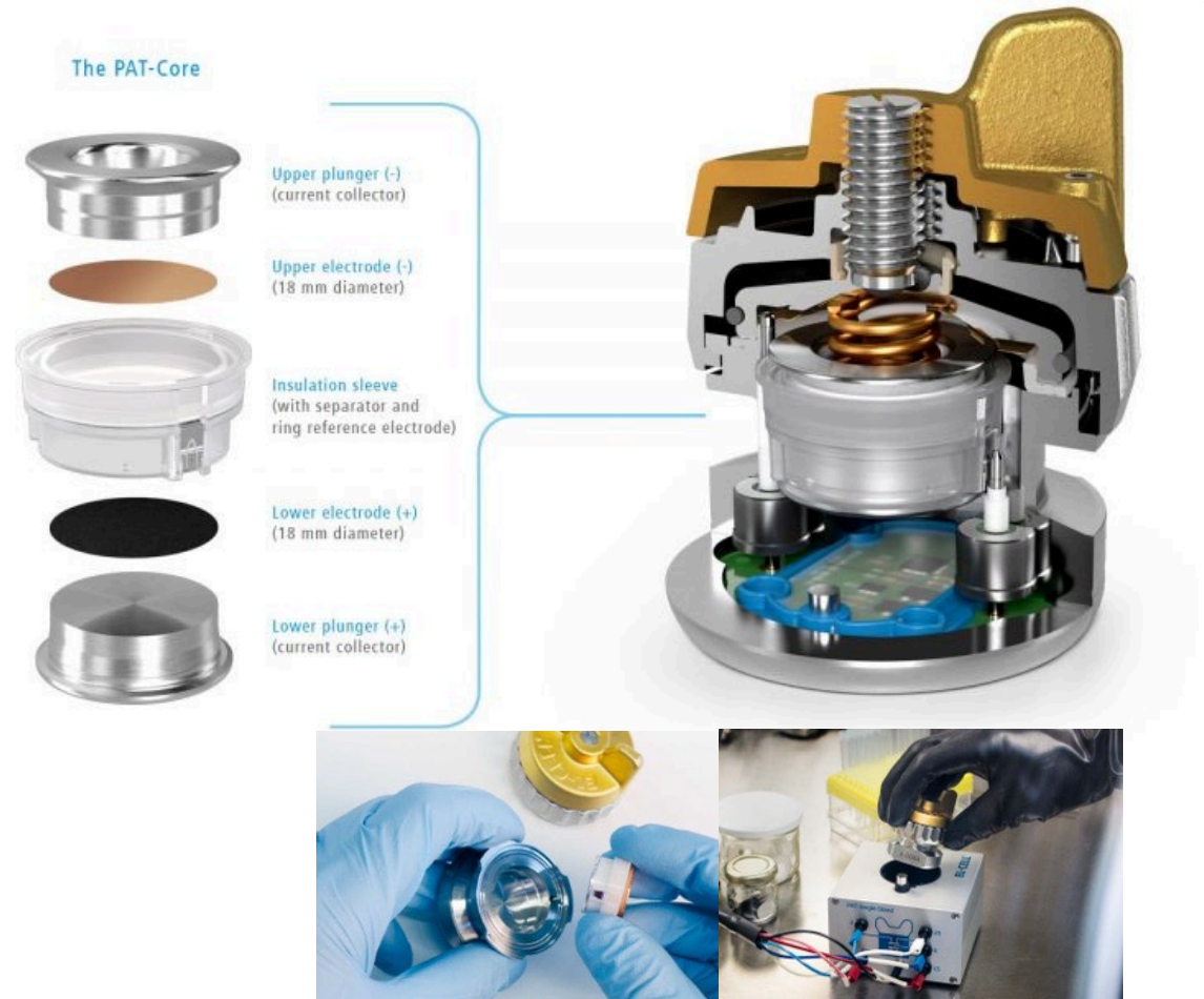
Scheme of EI-Cell used for testing (figures taken from el-cell.com).
